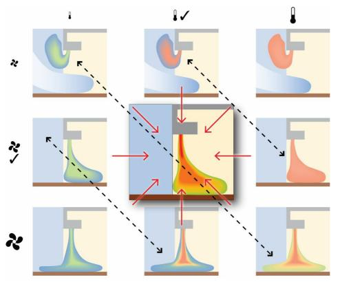
When set correctly, the air curtain always has sufficient strength to reach the floor (optimal climate separation) and always creates sufficient warmth to heat the incoming airflow to the required indoor temperature (comfort).
