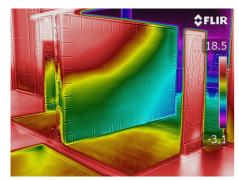
Air curtain off: significant air exchange
