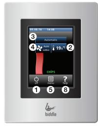
The auto-active control adjusts the air curtain fully automatically to all circumstances around the door. Without paying attention to the air curtain, the greatest possible comfort and least possible energy consumption are guaranteed.
