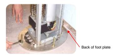
Using a hacksaw carefully cut the projecting bolts flush with the nut, ensuring the foot plate is not damaged or marked in any way.
