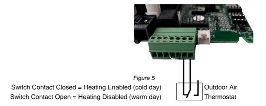
WARNING: Do not apply any voltage to terminal IN1 as this will damage the CCS PCB.
