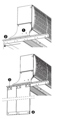
2.5 Installing the control box
